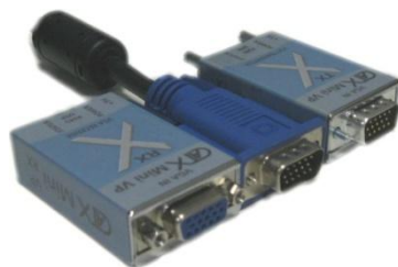
Comparison of CatX Mini Tx and Rx with a VGA connector
